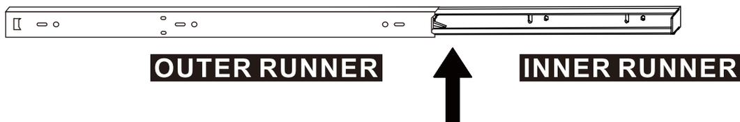
**EN\_Press** and hold the drawer runner lock and then continue to slide drawer runners apart, as shown.
