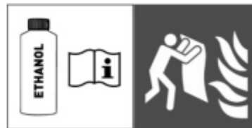
Adhere to instructions about fuel. ISO 7010-F016, Fire blanket
