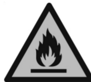
ISO 7010-W021, Warning; Flammable material
