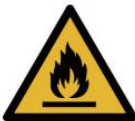
ISO 7010-W021, Warning; Flammable material
